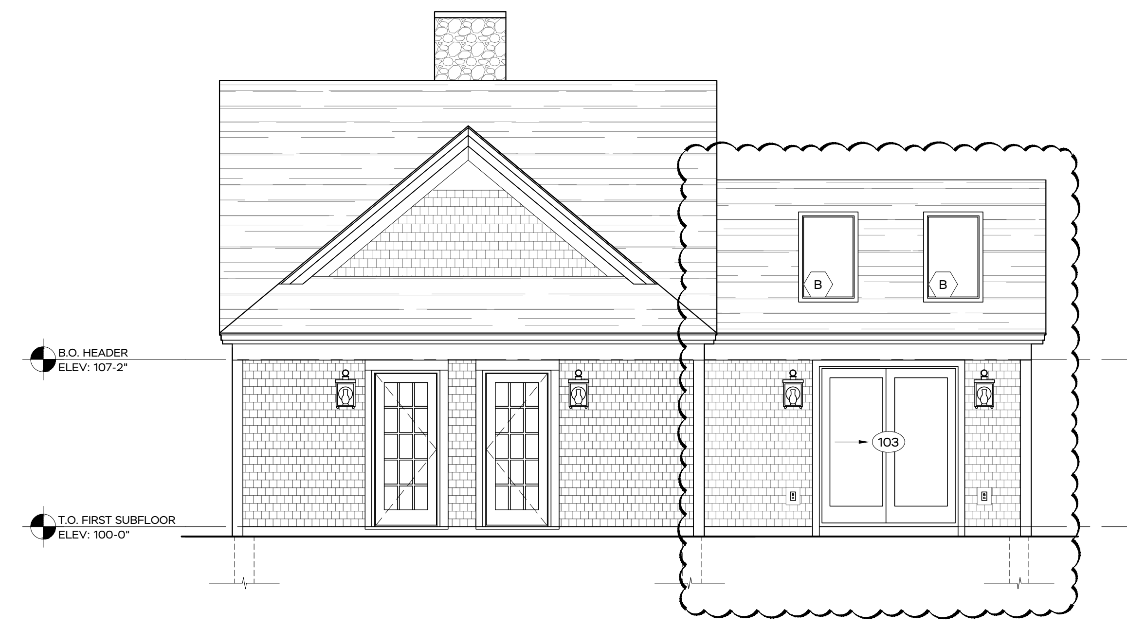
4 PROPOSED SOUTH ELEVATION SCALE: 1/4" = 1'-0"
