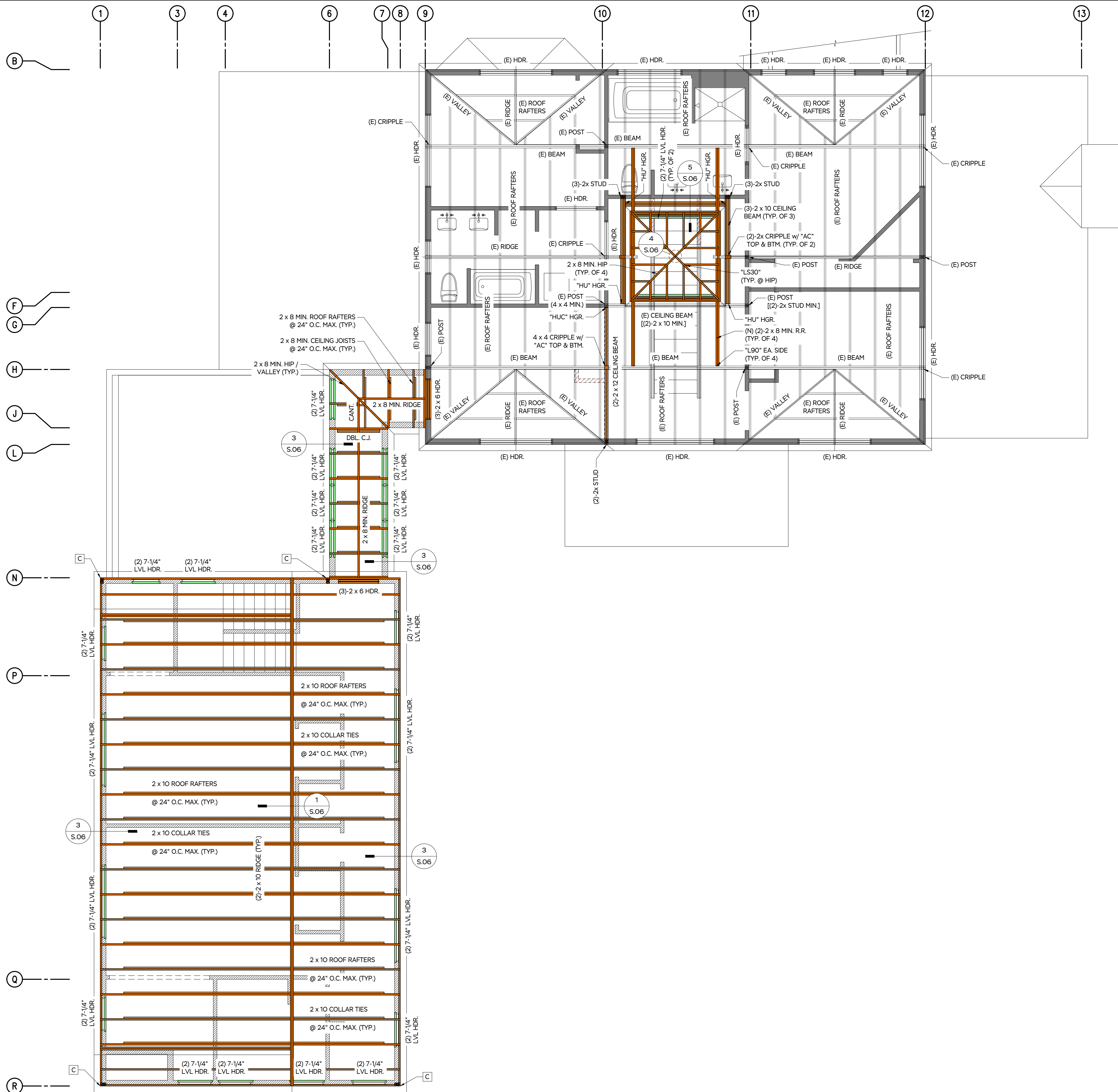
UPPER ROOF FRAMING PLAN VERIFY ALL DIMENSIONS WITH ARCHITECTURAL PLANS. SEE S.01 FOR NOTES AND SCHEDULES
