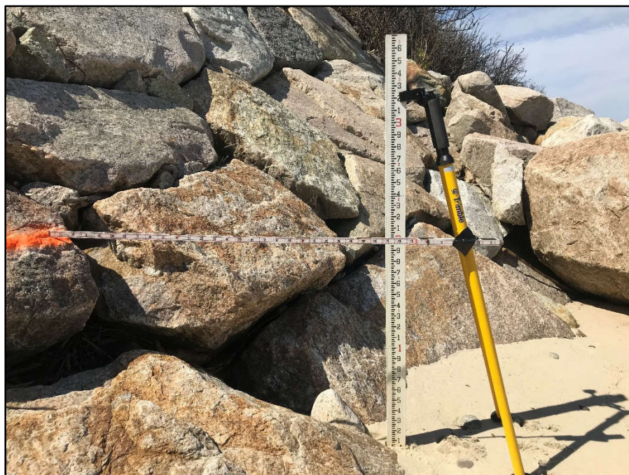
Monitoring Station #4: Beach at elevation 5.0 ft NGVD (2.0 ft below survey mark) on April 14, 2020.
