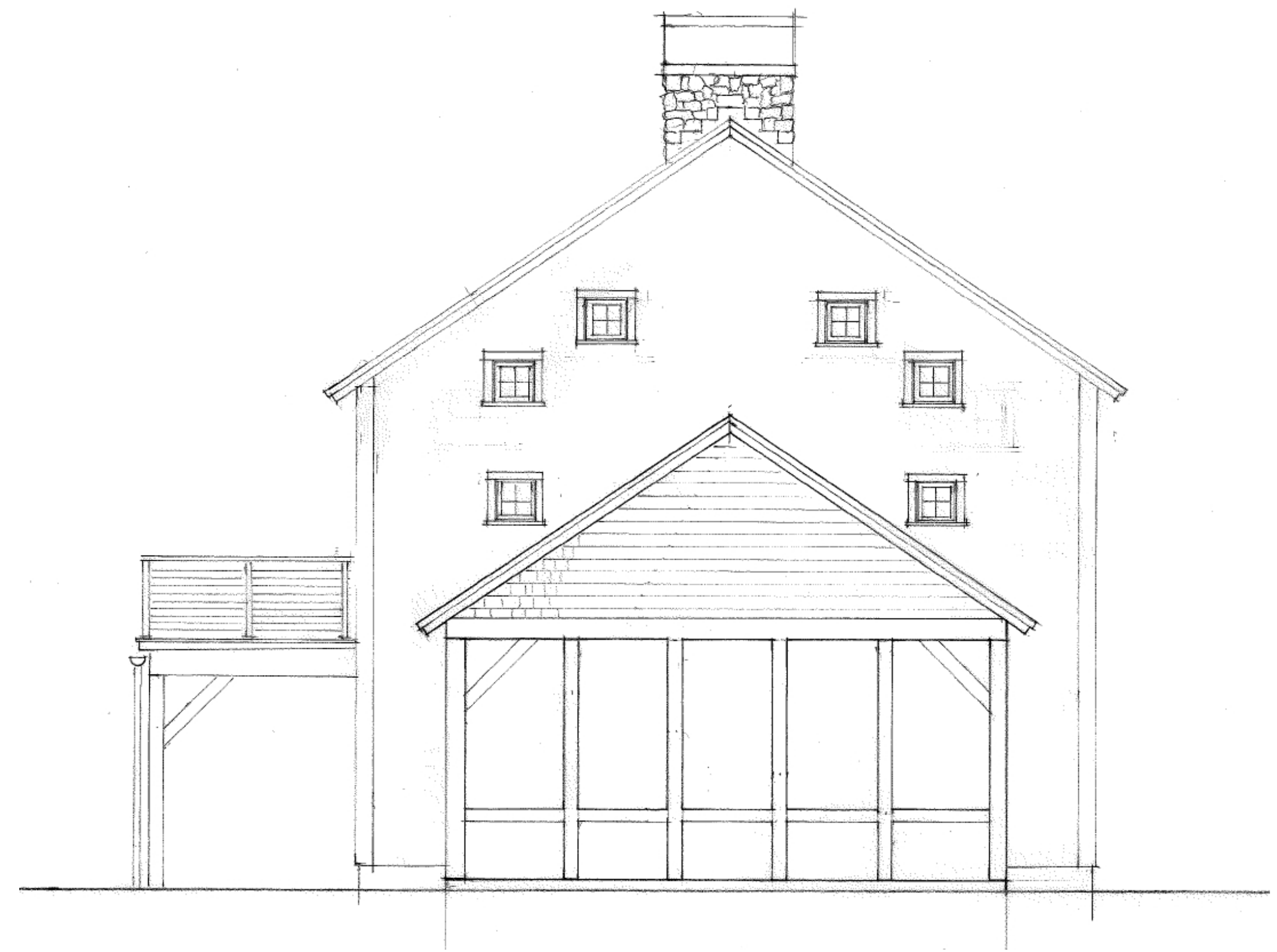
ELEVATION AT SCREENED PORCH 1/4"=1'-0"
