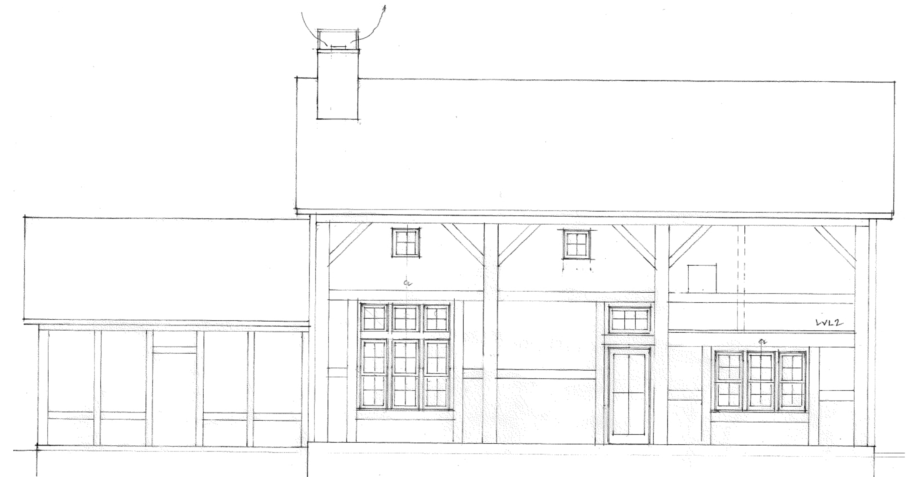
REAR ELEVATION W/ FRAME 1/4"=1'-0"
