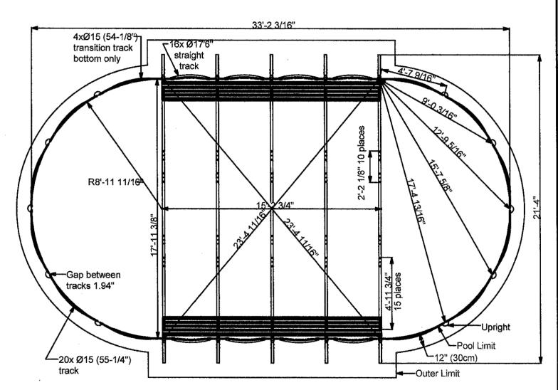
Perimeter 1043" (hole to hole)- Track length measured in track slot-All dimensions are in inches
