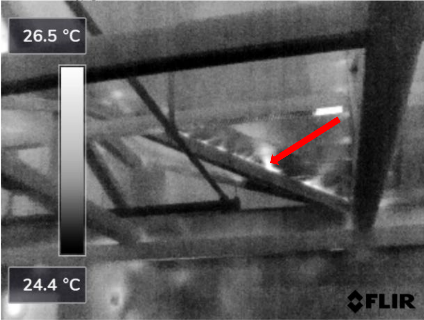
LIKELY AIR LEAKAGE AT ROOF VALLEYS
